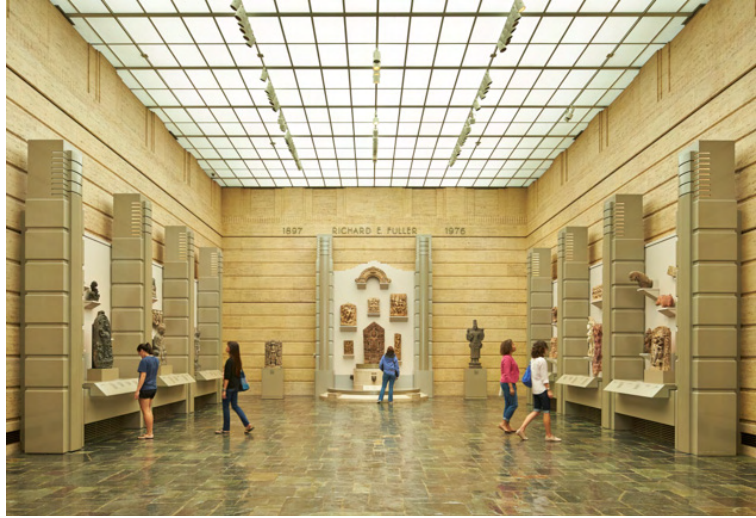
Figure 12. Translucent roofing panels provide for even, natural lighting in the Asian Art Museum in Seattle, Washington.
